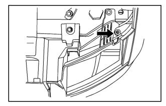
7. Locate the vertical headlamp aiming screws, which are under the hood near each headlamp assembly.
